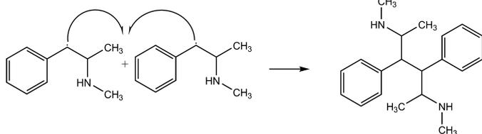
FIG. 13—Tentative mechanism for the formation of by-product 1 and by-product 2.
