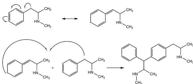
FIG. 14—Tentative mechanism for the formation of by-product 3.
